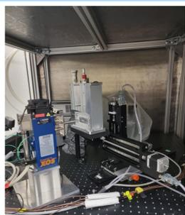
First tests on 20μm detectors were carried out on a compact X-ray generator (@ SuperXAS) with a Mo anode where the beam is focused with polycapillary optics to a 50 μm at 20 mm from the optics. A 2D scan with a 150 μm step size on the X axis and 40 μm on the Y axis was performed, acquiring 1000 frames (frame rate 2.5 MHz, exp. time 100 ns) of the 256 pixels at each position of the scan in dark and under illumination conditions in order to subtract the pedestal level from the data.
